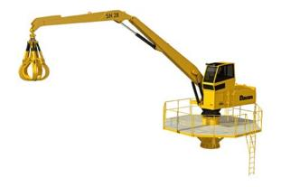
The SN 28 column-mounted loader is equipped with a grab (an excavator grab with a hinged mount) used to move scrap within its range of motion. The excavator is equipped with a HPD 05 -500.1 orange peel grab for this purpose.
