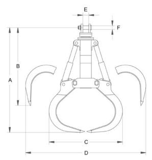
Hydraulic orange peel grab with open, half-closed or closed jaws. The basic model grab is delivered with a reliable hydraulic rotator, which is integrated into the upper part of the carrier.
