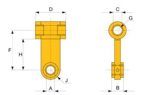
Hydraulic grab mounts are manufactured from St52 steel and the grab pin is mounted in two special sliding sleeves.
