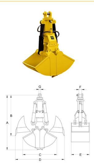
Hydraulic clamshell grab with rectangular jaws with a screwed split carrier. This configuration permits the use of various jaw models with different capacities while using a single grab carrier assembly. Combine different rectangular jaw assemblies of different capacities per this parameter sheet.
