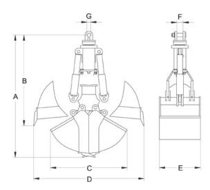
Hydraulic clamshell grab with rectangular jaws with a screwed split carrier. This configuration permits the use of various jaw models with different capacities while using a single grab carrier assembly. Combine different rectangular jaw assemblies of different capacities per this parameter sheet and curved jaws from the HCDK 17 line of all widths and volumes.
