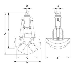
Hydraulic clamshell grab with curved jaws with a screwed split carrier. This configuration permits the use of various jaw models with different capacities while using a single grab carrier assembly. Combine different curved jaw assemblies of different capacities per this parameter sheet and rectangular jaws from the HCD 17 line of all widths and volumes.
