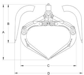
Hydraulic log grab in a claw design. The grab mechanism does not permit the elements to cross themselves and a two-row chain is used to provide clamping pressure when picking up smaller quantities of wood.
