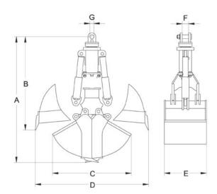
The MCD motorised hydraulic clamshell grab is a universal implement for loose materials. It is specifically intended for use on gantry crane slings or on similar lifting equipment.
