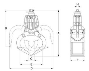
Hydraulic log grab in a claw design. This design allows logs to be gripped precisely along their axis. There is no need to take a full grab as the claw mechanism design permits overlapping as shown in the technical drawing at the bottom of this parameter sheet.
