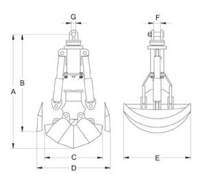
Hydraulic clamshell grab with curved jaws with a screwed split carrier. This configuration permits the use of various jaw models with different capacities while using a single grab carrier assembly. Combine different curved jaw assemblies of different capacities per this parameter sheet and rectangular jaws from the HCD 13 line of all widths and volumes.
