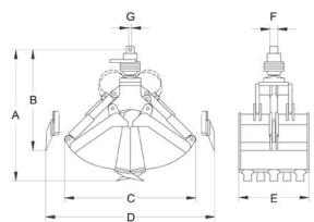
The hydraulic clamshell grab with rectangular jaws has an integrated carrier. The basic model grab is delivered with a reliable hydraulic rotator, which is integrated into the upper part of the carrier.
