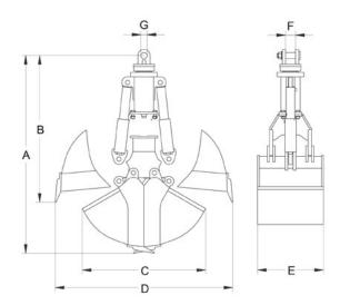
The hydraulic clamshell grab with rectangular jaws has an integrated carrier. The basic model grab is delivered with a reliable hydraulic rotator, which is integrated into the upper part of the carrier.
