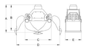
This universal hydraulic clamshell grab with rectangular jaws has an integrated carrier. The basic model grab is delivered with a reliable hydraulic rotator, which is integrated into the upper part of the carrier.
